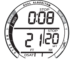
Fig. 28 - DECO STOP MAIN
